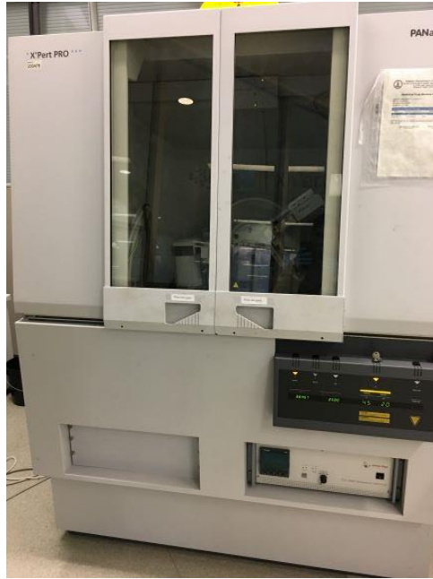
Figure 3. 7 XRD instrument used for an identification of phases in the samples.
