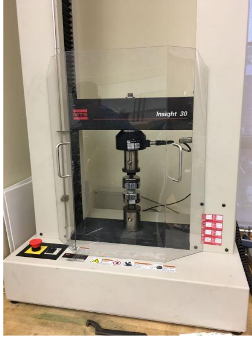
Figure 3. 5 MTS Model Insight 30 Capacity used for the compressive strength test.
