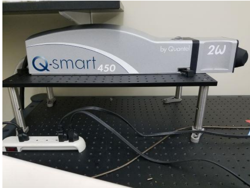
Figure 4. 1 Picture of the Q-smart 450 Nd:YAG laser used in this work.
