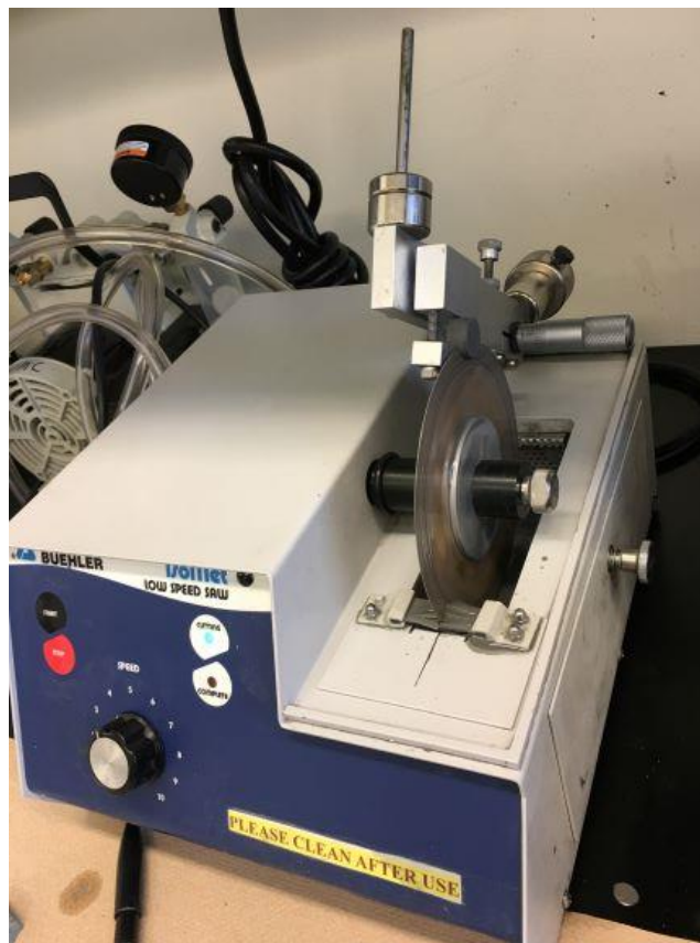
Figure 4. 4 IsoMet™ low speed precision cutter.
