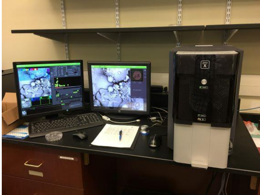
Figure 3. 9 The Phenom ProX desktop SEM with EDX.
