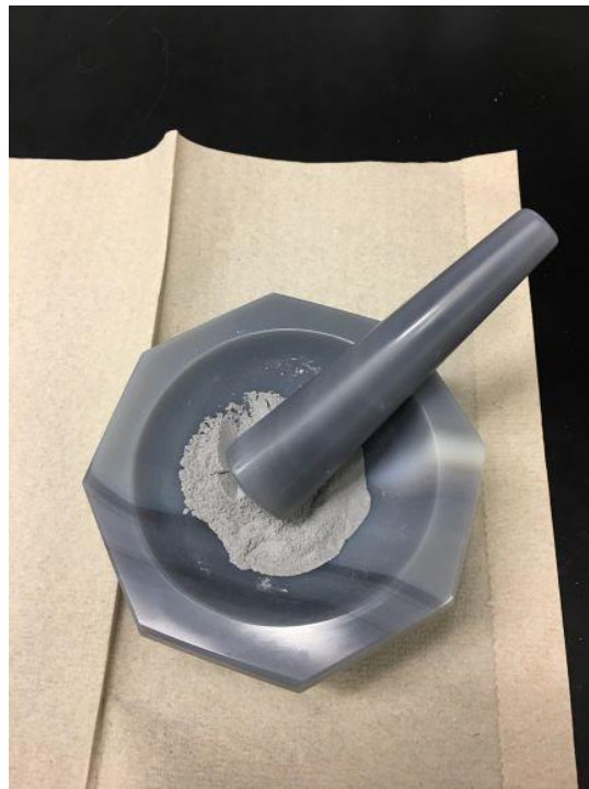
Figure 3. 6 The mortar and pestle used for grinding samples for XRD.
