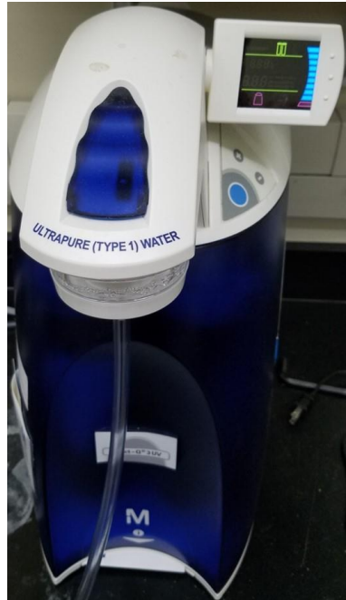
Figure 3. 1 Millipore Direct-Q® 3 UV Water Purification System used for obtaining DIW.
