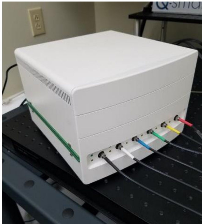
Figure 4. 2 Picture of Aurora LIBS spectrometer used in this work.
