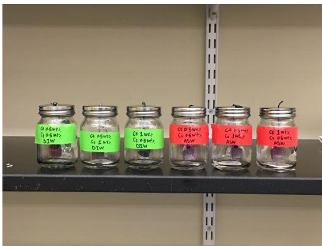
Figure 5. 1 Suspended RCS waste form during leaching test.
